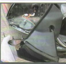
7.Replace the new bend lamp and restore the installation screws and connectors
