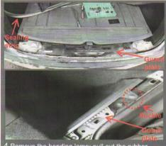
4.Remove the bending lamp: pull out the rubber sealing strip, use the prying plate to remove the guard plate, pry off the snap on the figure, and then take out the storage partitions on both sides
