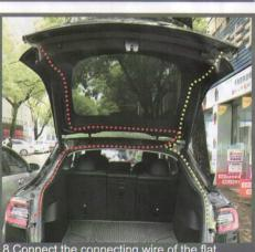
8.Connect the connecting wire of the flat bending lamp as shown in the figure and tie it with rolling tape
