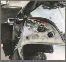
2.Remove the flat lamp: Unplug the connector, unscrew the screw (above), and remove the flat lamp with the rocker (below)
