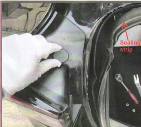
4. Remove the bending lamp: unscrew the fixing part of the bending lamp and pull out the rubber sealing strip
