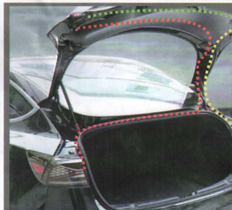
8. Connect the connecting wire as shown in the figure and tie it with rolling tape
